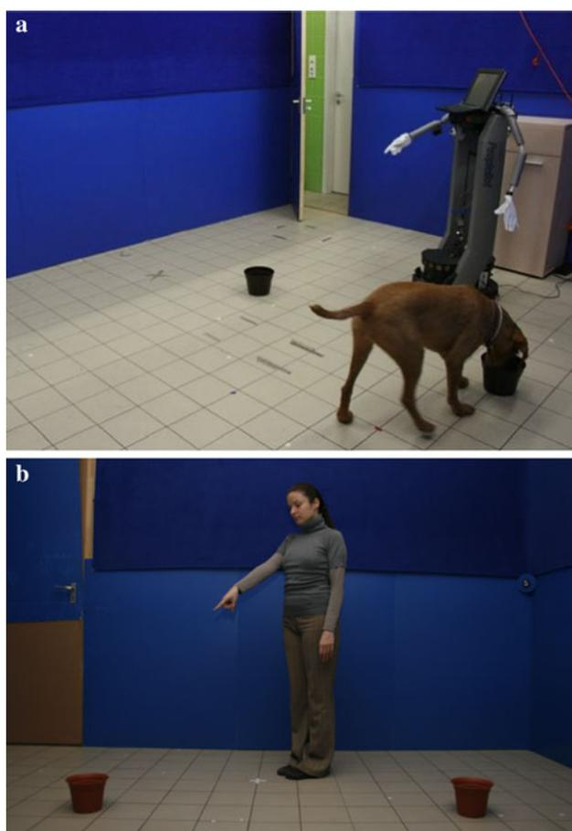
**Fig. 1** **a** The customized PeopleBot mobile platform, which was equipped with a 5 degree of freedom robotic arm endowed with a four-fingered hand. **b** The human experimenter adjusted her movements to the physical abilities and constraints of the robot. The robot had only one moveable pointing arm, and thus, the human experimenter always used the same arm for pointing
