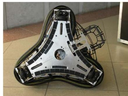
Figure 4. The robot omniwheels
