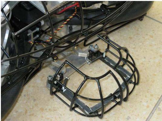
Figure 7. The gripper
